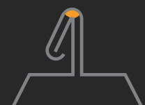
Compressed Field Seam and Snap-Together
