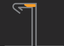
Compressed Field Seam and Snap-Together
