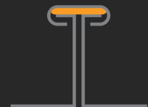
Compressed Field Seam and Snap-Together
